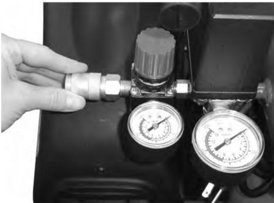
**Figure 3.** Installing the Air Chuck
