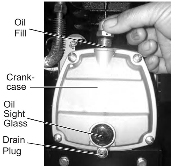
**Figure 2.** Installing the Oil & Oil Breather Cap
