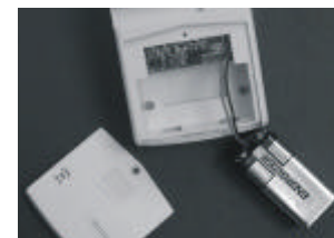
Insert 9V alkaline battery to the sensor
